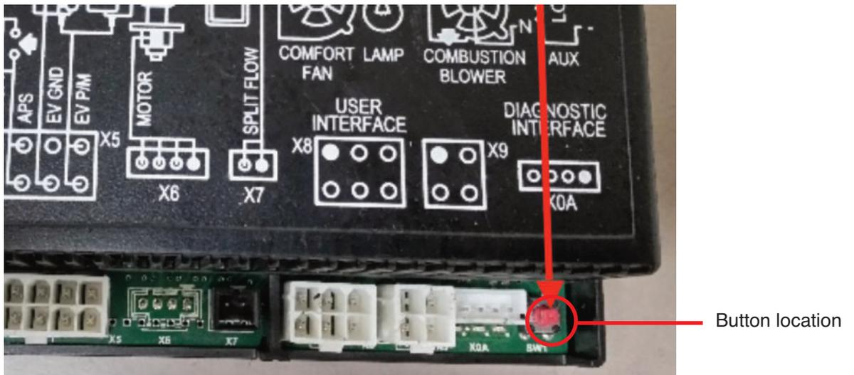
5. Press the on button on the remote – four beeps should be heard.
