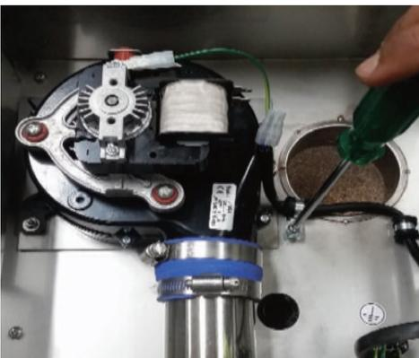
Push fan terminal into position. And affix to wall.
