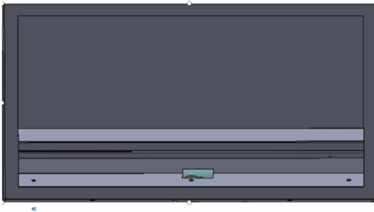
Locate side trays on either side of the firebox. Ensure that they are sitting flush against the side walls and screw them in from the front (if the trays do not sit flat then use the rear screw holes to screw them down).
