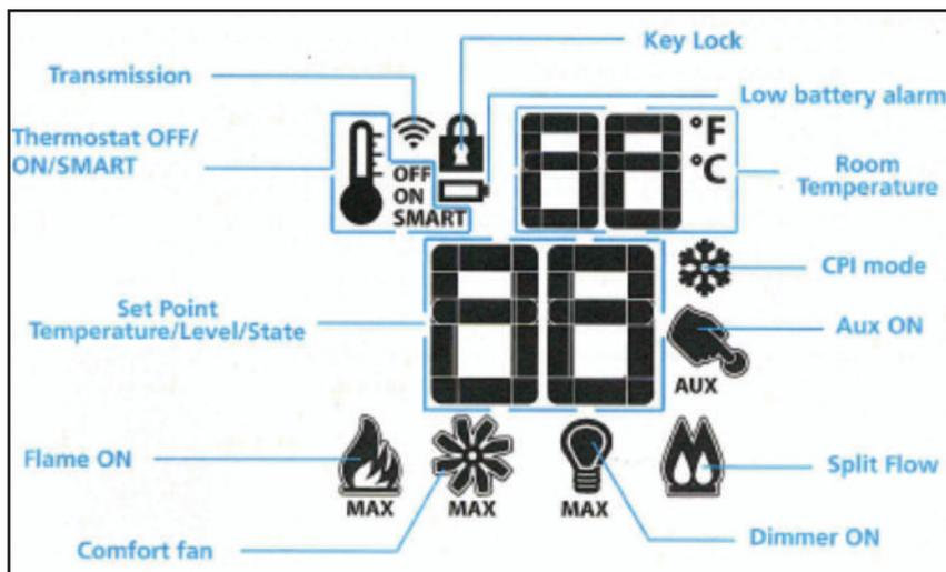
Transmitter LCD display
